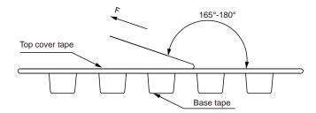
The peel force of top cover tape shall be between 0.1 to 1.17 N
