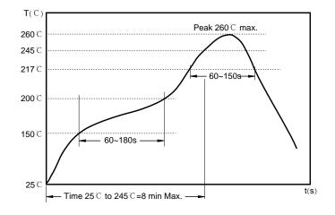
Preheat condition:  $150 \sim 200 \degree$  /  $60 \sim 180$  sec. Allowed time above  $217\degree$  :  $60 \sim 150$  sec. Max temperature:  $260\degree$  . Max time at max temperature: 10 sec.
