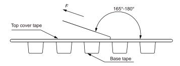
The peel force of top cover tape shall be between 0.3 to 1.17 N
