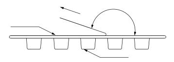
The peel force of top cover tape shall be between 0.14 to 0.78 N  $\,$
